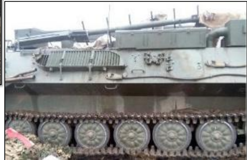
R-378B tracked jammer - one part of the R-330 Mandat complex. Source: © 10 August 2016, Informnapalm.org 106
