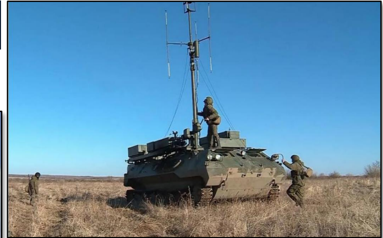
R-934BMV jamming station - one part of the RB-310B Borisoglebsk-2 complex. Source: © 14 September 2022, Gagadget 153
