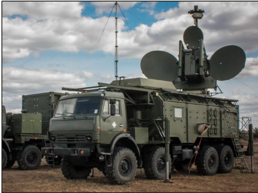
1L269 Krasukha-2 and 1RL257 Krasukha-4 systems deployed with the army's independent EW brigades to jam airborne radars. Source: © 26 May 2022, ADBR 26
