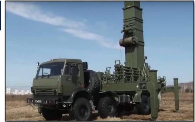
KamAZ 530501 8x8 military truck with the extendable antenna mast.
