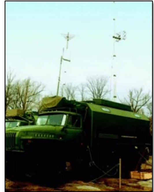
R-330K control point module, functioning as part of the R-330 Mandat EW complex. Source: © 31 May 2023, Armed Conflicts 103
