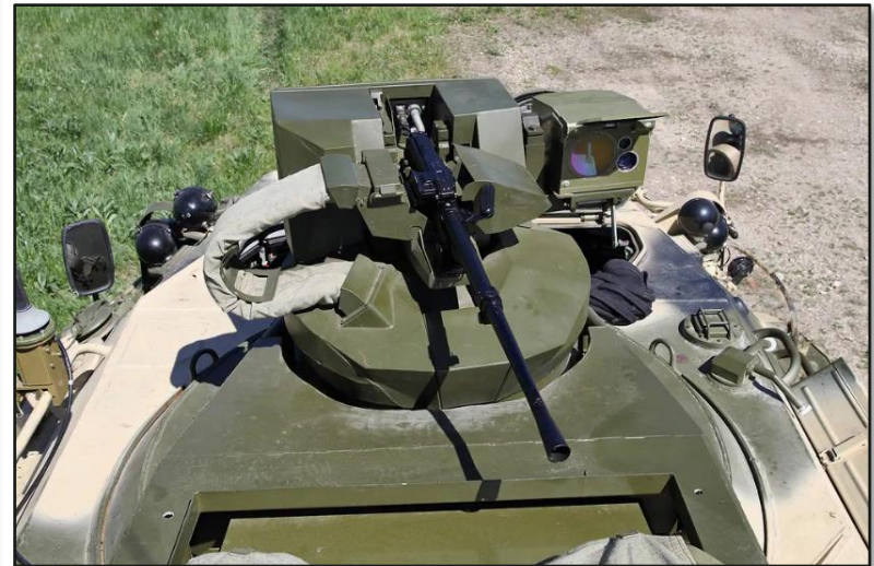
Remotely controlled combat module with a PKT machine gun.
