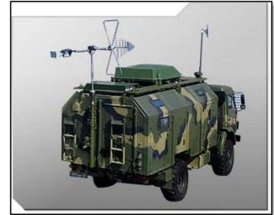
RB-636AM2 Svet-KU mounted on KamAZ-4350 two-axle chassis. Source: © 25 October 2017, Defense Express 171
