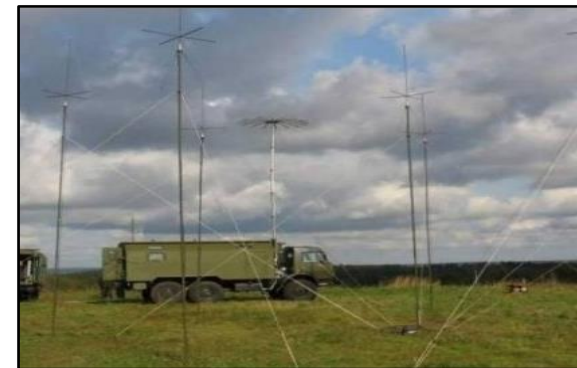
TORN automated jamming complex fully deployed with supporting antennae.
