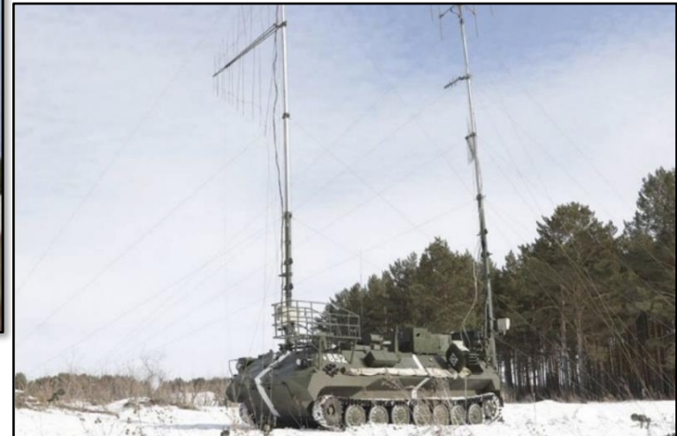
R-330BMV jamming station - one part of the RB-310B Borisoglebsk-2 complex. Source: © 14 June 2019, Janes 154
