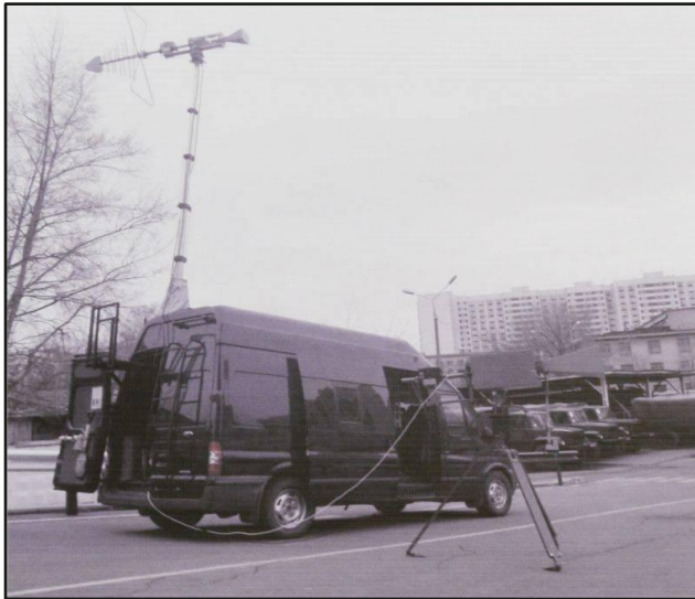
Deployed RB-636AM2 Svet-KU complex - Newer variant based on the Ford Transit chassis. Source: © 19 October 2015, Topwar.ru 174
