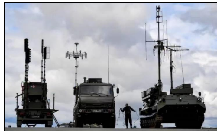
The Tirada complex includes a mobile command center, a hardware machine with means of detecting communications and jamming – mounted on a KamAZ chassis, and an electric generator. Source: © 9 October 2022, For-ua.info 211
