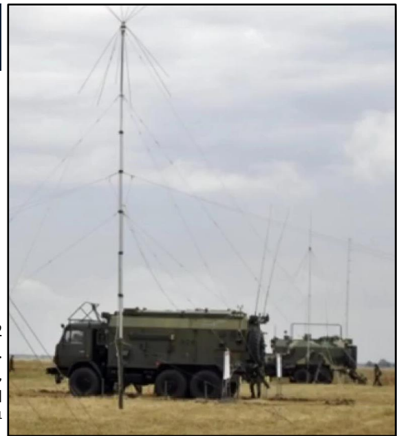
Right: Mobile Tirada-2 satellite jamming systems. Source: © April 2021, Center for Strategic and International Studies 221
