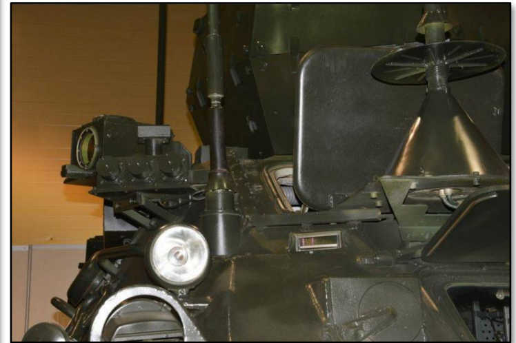
Auxiliary antenna, optoelectronic sensor, and grenade launcher on starboard side of RB-531 Infauna. Source: © 15 October 2015, Topwar.ru 167
