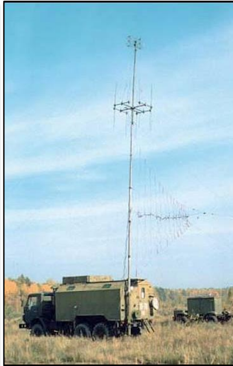
Deployed configuration of the KamAZ hosted R-330T. Source: © 1 May 2009, Air Power Australia 115
