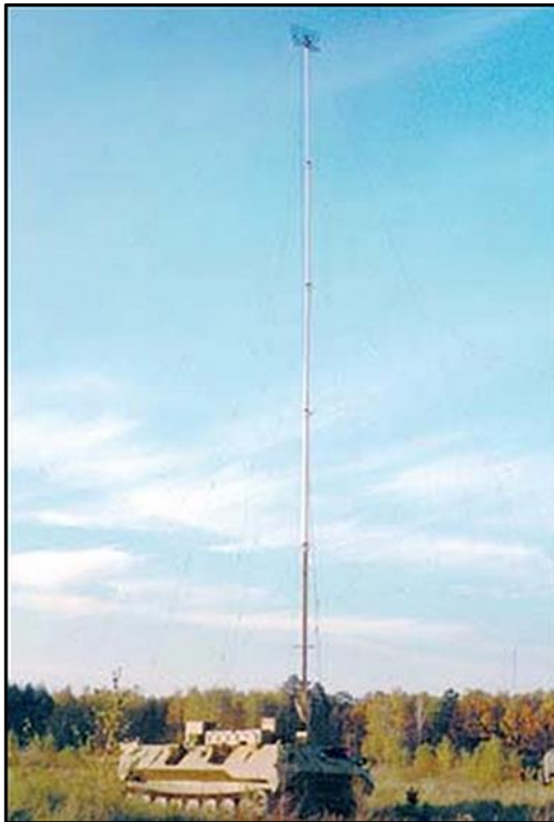
Deployed configuration of the MTLBu hosted R-330B tracked chassis. Source: © 1 May 2009, Air Power Australia 115
