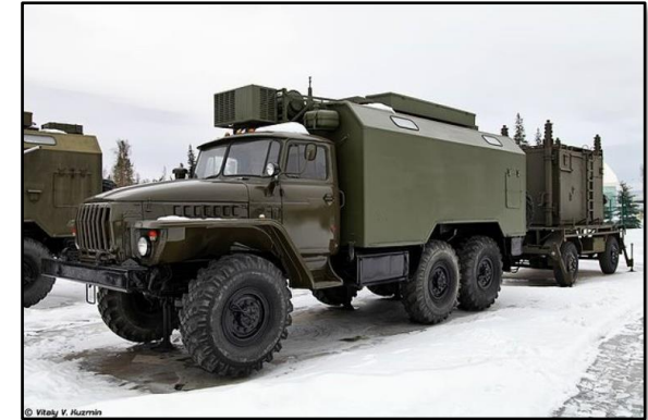
R-330Zh jamming station - one part of the R-330M1P Diabazol jamming complex.
