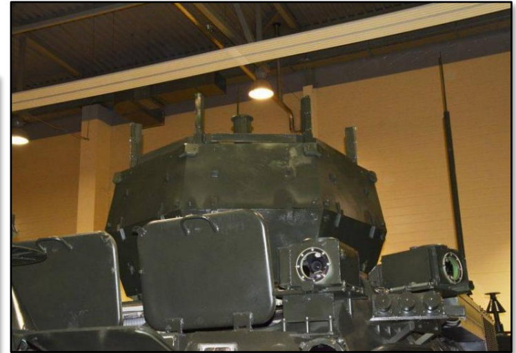
Roof-mounted dome antenna housing on the RB-531B Infauna. Source: © 15 October 2015, Topwar.ru 167
