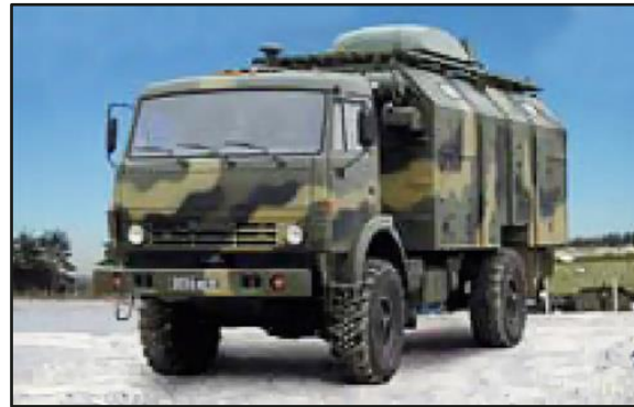
Mobile radio monitoring complex "Svet-KU« on KamAZ brand chassis. Source: © 04 May 2014, militaryrussia.ru 175
