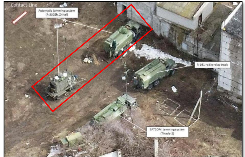
R-330Zh Zhitel station (red) alongside Tirada-2 jammer. Source: © 3 April 2019, UNIAN 121
