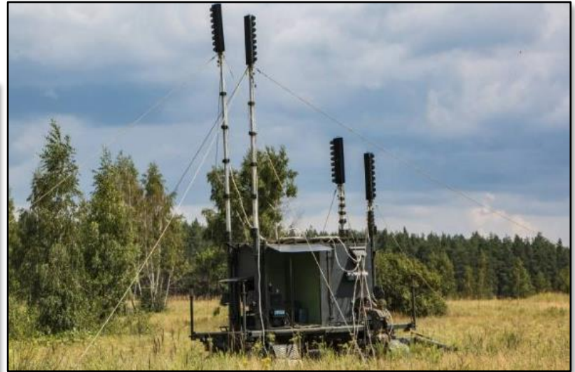
R-330Zh Zhitel antenna reconnaissance and suppression module in field deployment. Source: © 26 July 2016, Topwar.ru 120
