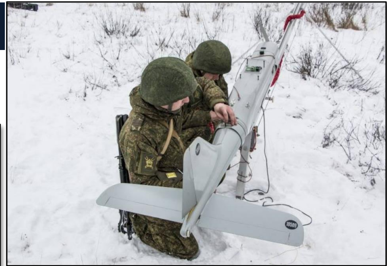
Orlan-10 drone loaded onto launch catapult as part of Leer-3 system. Source: © 21 February 2018, Topwar.ru 158
