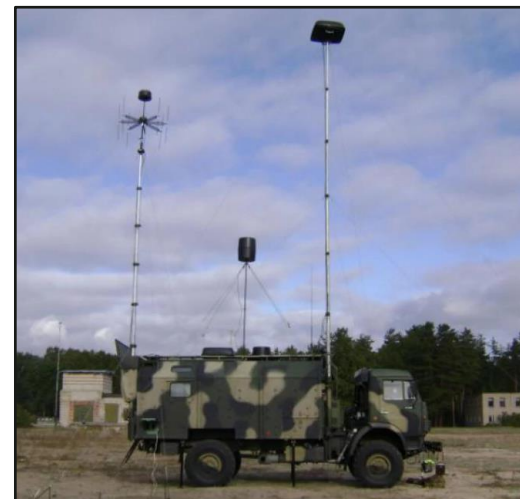
Mobile automated complex of electronic warfare (EW) MKTK-1A "Judoist" Source: © Date accessed: 6 June 2023, ВПК 71
