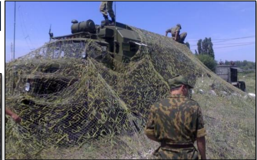
R-325U high frequency jammer under camouflage netting - part of the R-330 Mandat complex). Source: © 15 July 2011, ruqrz.com 105
