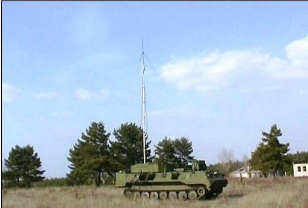
R-330KMV - modernized version of R-330K used in R-330 Mandat complex. Source: © 28 May 2015, Twitter 152
