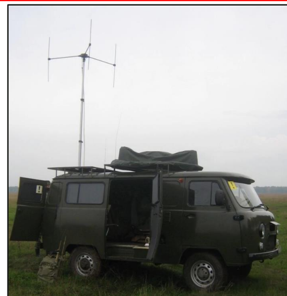
RP-377L/LA Lorandit-M on UAZ chassis. Source: © 3 12 April 2014, Live Journal 187
